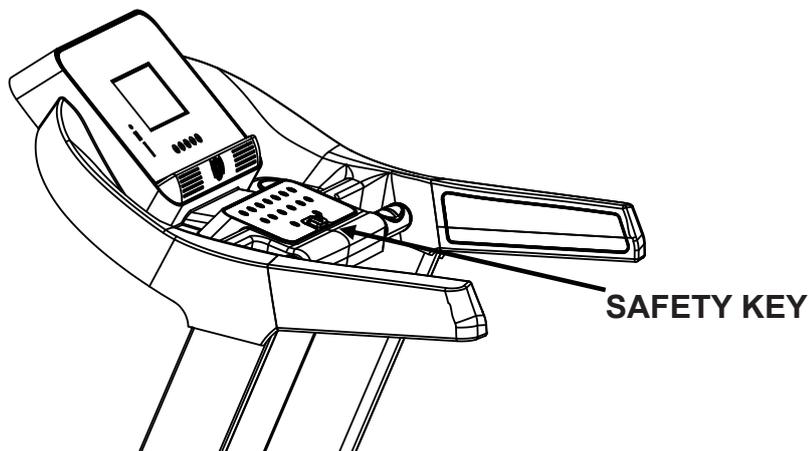
Before beginning a workout session ensure that the Safety Tether Key is properly placed onto the Computer Console and the Safety Clip is securely attached to an article of your clothing. If you fall the clip will pull out the SAFETY KEY from the Computer Console and the running belt will stop immediately for emergency stop, helping to prevent injury.
