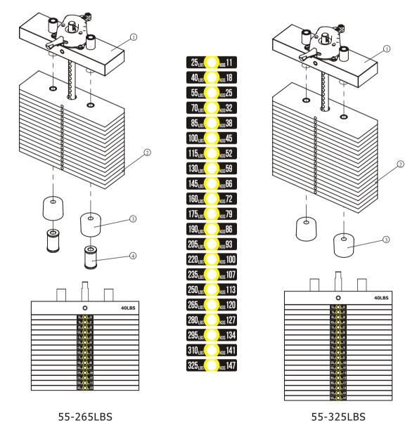
Weight plate sticker paste schematic diagram
