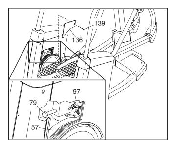
Next, loosen the Pivot Screw (97), tighten the Belt Adjustment Screw (79) until the Drive Belt (57) is tight, and then retighten the Pivot Screw.
