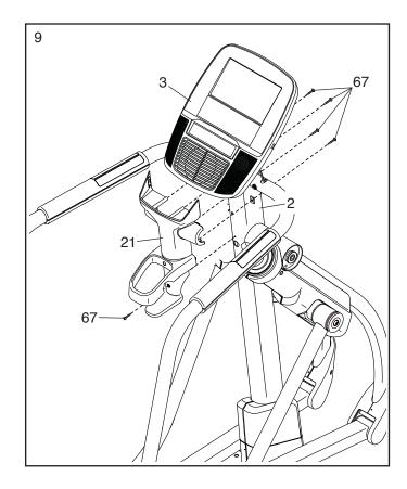
Press the tabs on the Front Upright Cover (20) into the Rear Upright Cover (21). Then, attach the Front Upright Cover to the Upright (2) with an M4 x 16mm Screw (67).
