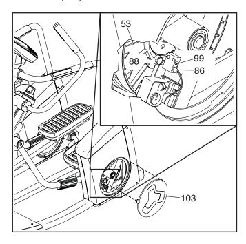
Next, locate the Reed Switch (86). Move the pedals until one of the Magnets (88) on the Pulley (53) is aligned with the Reed Switch. Then, loosen the M5 x 16mm Flat Head Screw (99), slide the Reed Switch slightly toward or away from the Magnet, and retighten the Flat Head Screw.
